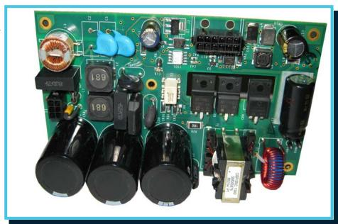
terconnection is accomplished using two vertically mounted TE connectors. The **AC20W-12V-500-PBF** is designed and manufactured to stand-up to the harsh operating environments encountered in today's aircraft installations.
