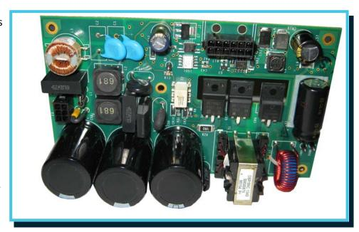
hold-up capacitors; in this area maximum height is less than 1.26". Interconnection is accomplished using two right angle Molex connectors. The **AC20W-48V** is designed and manufactured to stand-up to the harsh operating environments encountered in today's aircraft installations.
