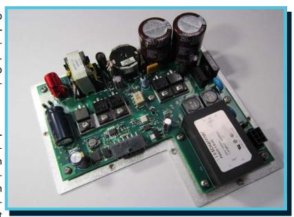
of header type connectors. The **AC30W-48V-PBF** is designed and manufactured to stand-up to the harsh operating environments encountered in today's aircraft installations.
