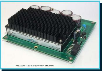
**PBF** is constructed on a multi-layer PWB occupying ~34in<sup>2</sup>. Component height is less than 1.26" with integral finned heatsink. Interconnection is accomplished using Samtec IPBT connectors. The **MS100W-12VE-5V-500-PBF** is designed and manufactured to stand-up to the harsh operating environments encountered in today's aircraft installations.
